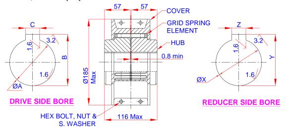
Tolerance for untolerenced dimensions are as per Medium Class of **IS 2102 Part I** (latest revision).
