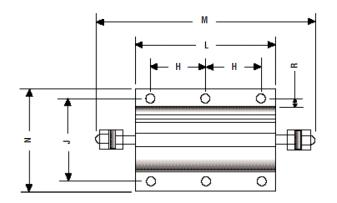
6 x Mounting Hole HSC200 - 5.3mm HSC250 - 5.3mm HSC300 - 6.5mm
