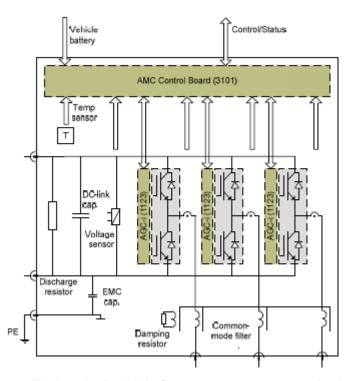
The damping resistor will absorb the high frequency components in the inverter output generated as a result of IGBT switching. A ferrite core assembly is provided at the output of the auxiliary inverter which will trap the high frequencies which are dissipated by the damping resistor.
