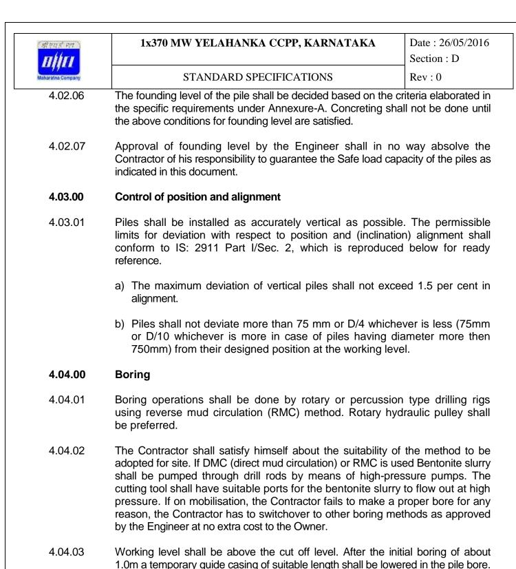
The diameter of guide casing shall be of such diameter, so as to give the necessary finished diameter of the concrete pile. The centre line of guide casing shall be checked before continuing further boring. Guide casing shall be minimum of 1.0m length. Additional length of casing may be used depending
