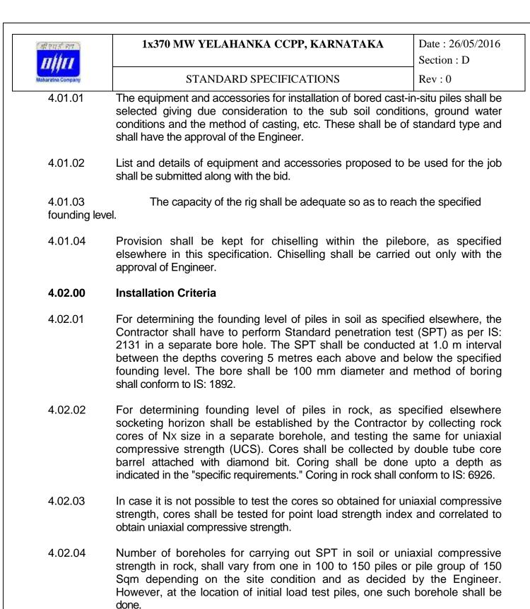
A protocol between contractor and BHEL site shall be maintained regarding the strata at founding level. SPT value and UCS from the nearest borehole shall
