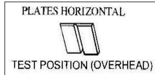
Figure A6.8 Overhead Position
