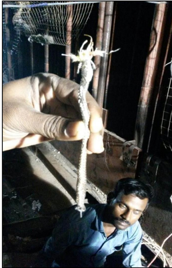
Figure B4.2: K - Type Thermocouple
