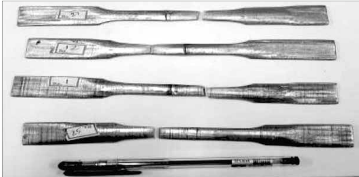
Figure 3 - Tensile test specimen – Failure location at base metal
