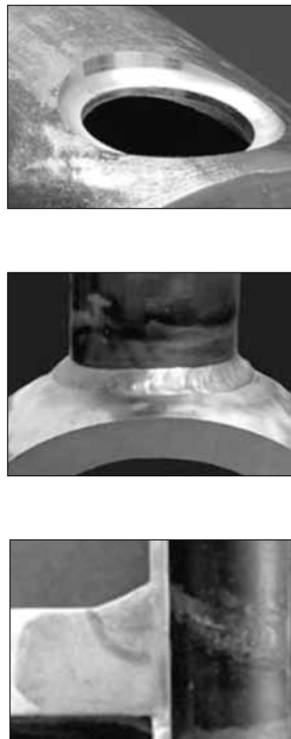
Figure 3 (a, b, c) - Stick-through with standard J bevel groove design
