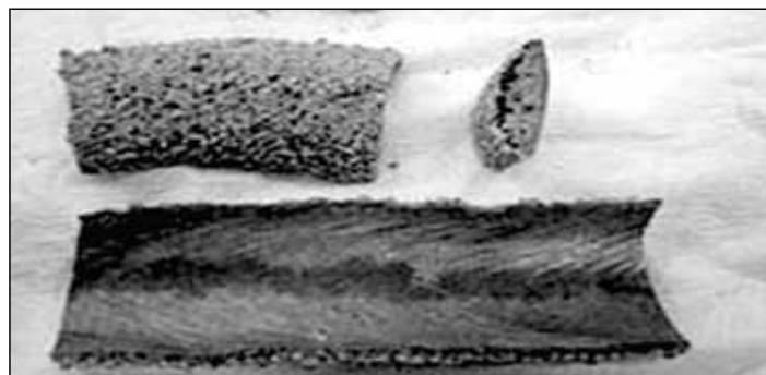
Figure5 - Welding slag formed with high basic fluxes
