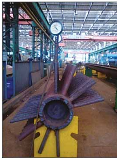
Figure 7 - Hydro test on mock up header
