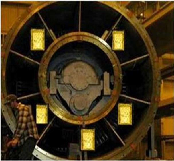
Figure 4. Exhaust Diffuser with VpCI Pouches
