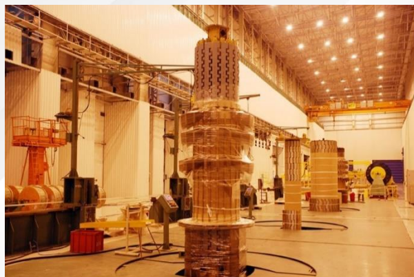
Transformers - Vertical Winding Machine
