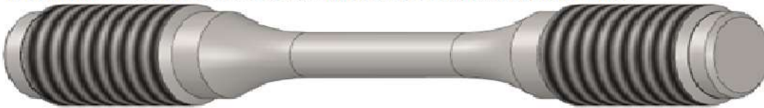
Figure 2: Low Cycle Fatigue testing M12 sample drawing
