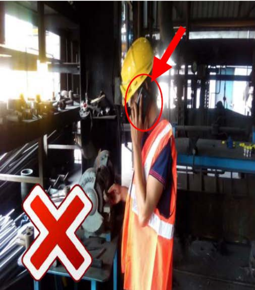
E. Operating Grinding machine
