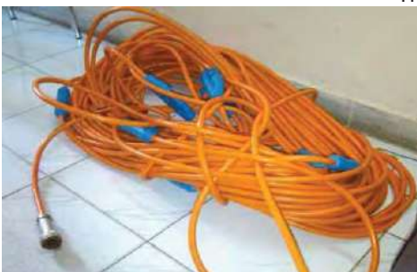
24 Channel Seismic Cable
