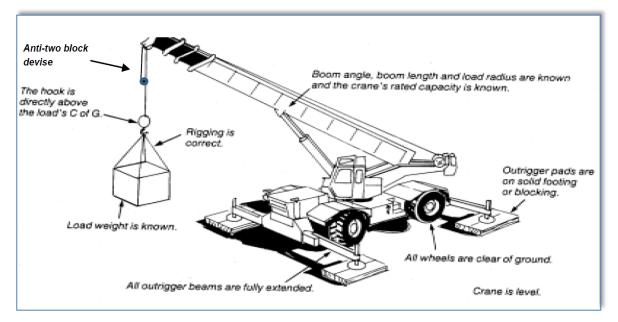
Fig. 5.2 Proper Crane Setup
