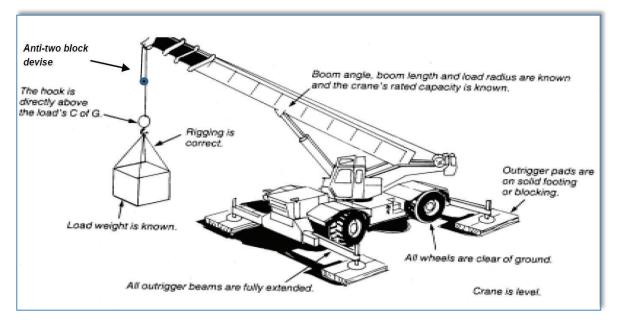
Fig. 5.2 Proper Crane Setup
