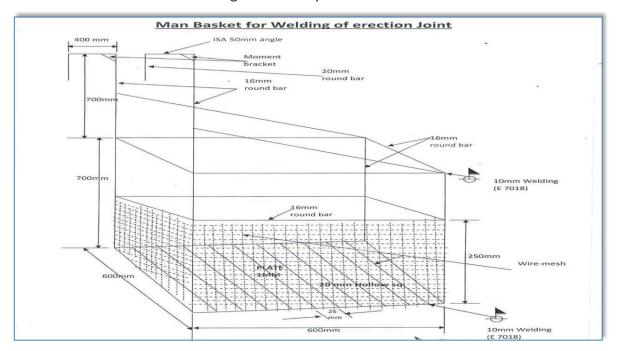
Fig. 5.1 Man Basket for Welding Erection Joint
