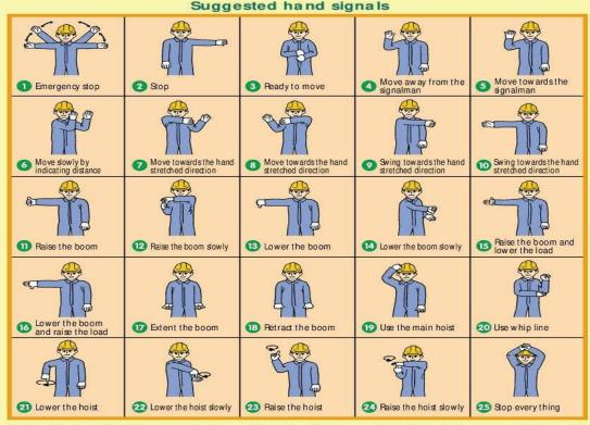
Note: During the lifting operation, either the slinger or signaller shall communicate with the operator. Other communication methods (e.g., wireless walkie-talkies, telephones, etc.) may also be used.
