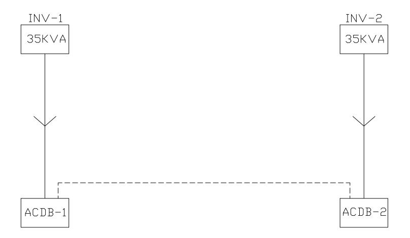
NOTE: FEEDER DETAILS OF ACDB ATTACHED IN THE FEEDER LIST
