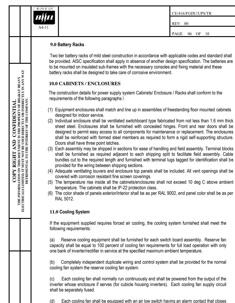
upon failure of air flow or rise of temperature.
