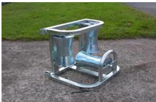
5. Pulley: May used for cable lifting in raise or cable shaft
