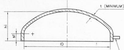
t =MIN. THICK OF DISHED END AFTER FORMING.
