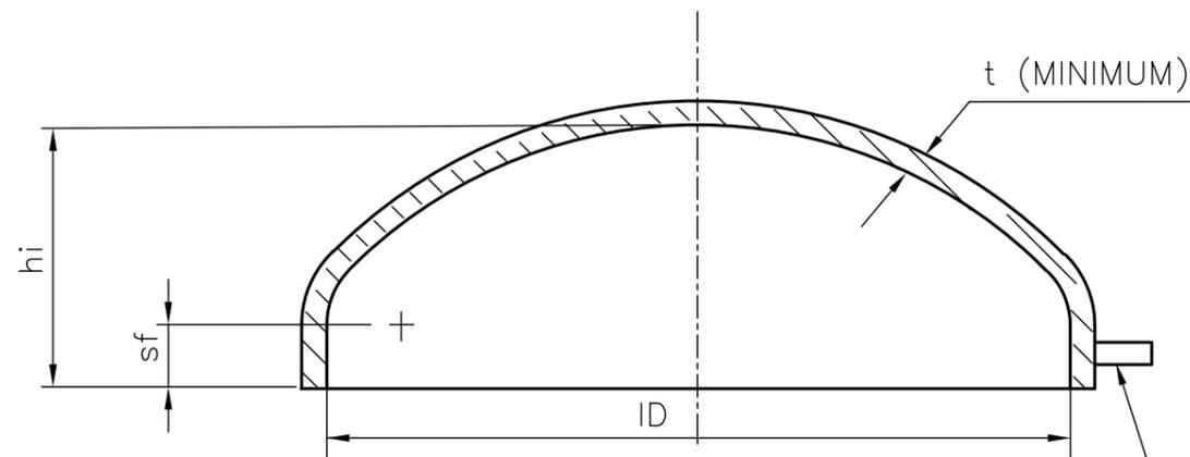
**t** = MIN. THICK OF DISHED END AFTER FORMING.
