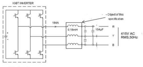
IGBT switching frequency= 2 to 4 KHz Output frequency= 50Hz
