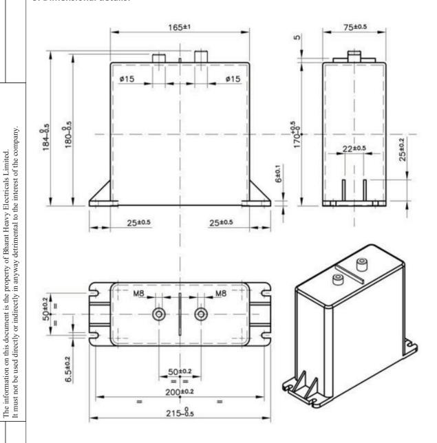
Terminals: M8X10, Maximum Tightening torque: 12Nm
