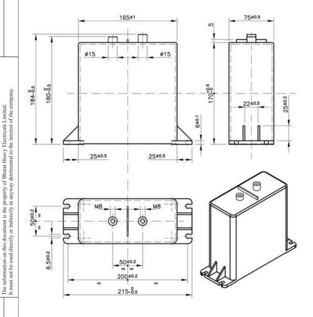
Terminals: M8X10, Maximum Tightening torque: 12Nm
