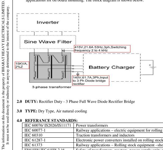
2.0 DUTY: Rectifier Duty - 3 Phase Full Wave Diode Rectifier Bridge
