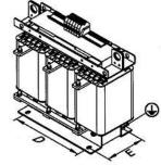
Dimensions in mm A= 450; B=235; C=440; D=316; E=173 F=140; G=22 Mounting hole = Φ12x18
