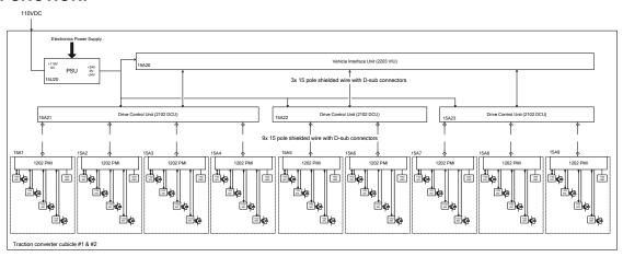
The power supply receives 110V DC from the locomotive battery and generates 24V out of that for powering up the control circuit of traction converter. The Temperature classification of the electrolytic capacitors used in power supply is 105°C.
