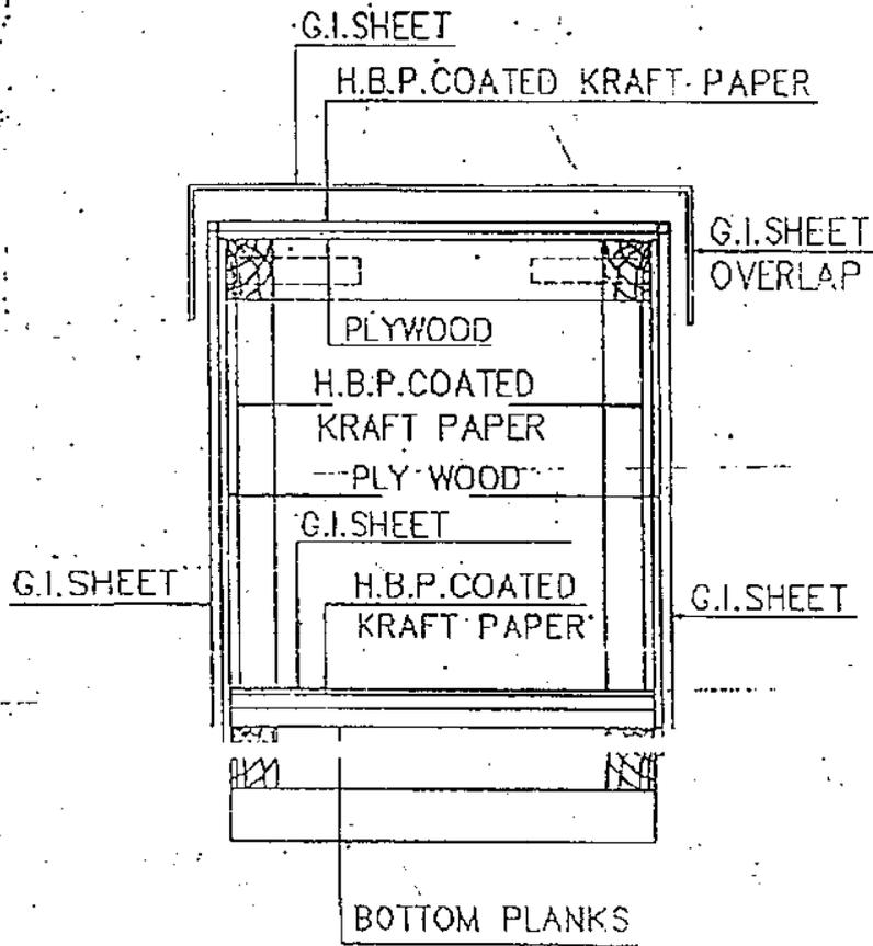
FIG-16 : CLOSED PACKING CASE WITH G.I.SHEET
