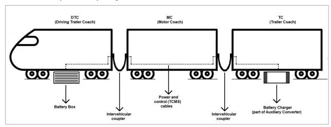
Distance between Battery box and battery charger is 60 meter approx.
