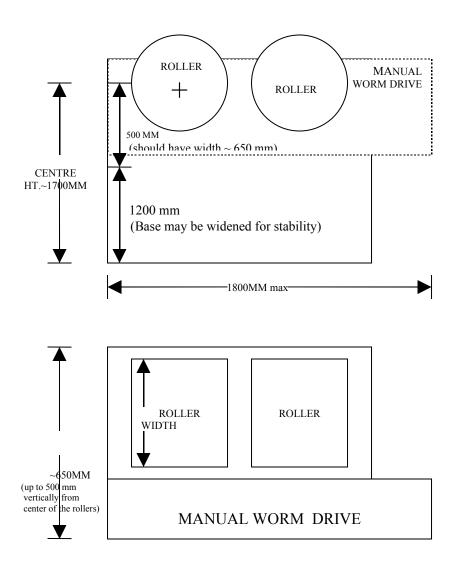
PROPOSED SCHEMATIC DIAGRAM OF EACH END SUPPORT OF 100 T ROTATOR (EACH SET CONSISTS OF ONE END SUPPORTS WITH WORM DRIVE AND THE OTHER WITHOUT WORM DRIVE)
