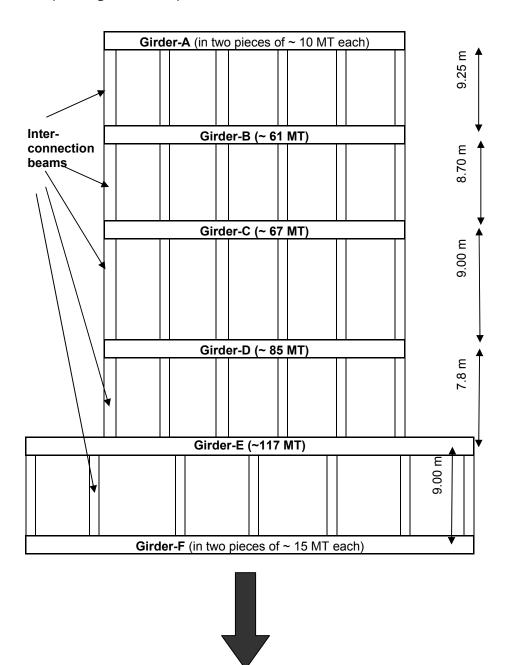
Direction of Crane Movement for erection of Boiler Ceiling Girders & Interconnection Beams
