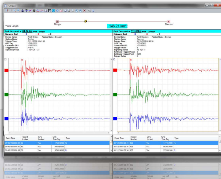
Viewer showing TWS waveforms from each end of the line for a line fault
