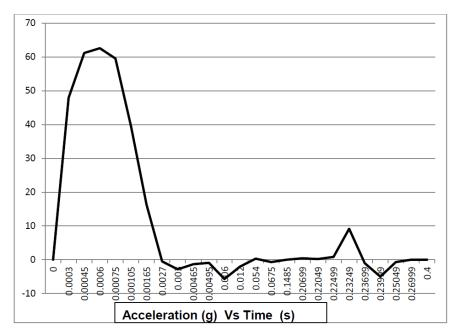
If the supplier has performed a shock load test on a pressure compensator of similar design, the corresponding test report shall be submitted for review and scrutiny. In the event that the supplier is unable to perform the shock load test, a structural analysis report using Finite Element Method (FEM) software shall be provided. This analysis must demonstrate the pressure compensator's compliance with the specified shock load requirements.
