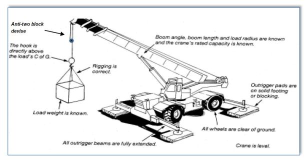
Fig. 5.2 Proper Crane Setup
