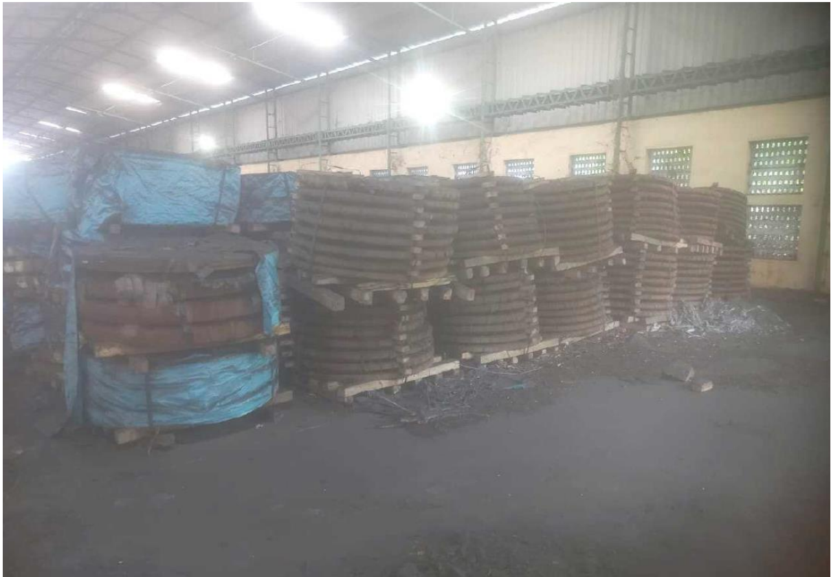
SFW SHED Outside ( CS Strips IS 513 Gr EDD & SS Strip SA 240 Type 409)
