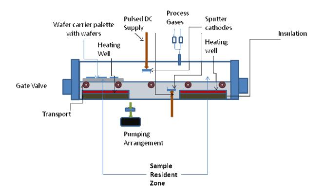
Fig. 5 Schematic of ITO Deposition Chamber
