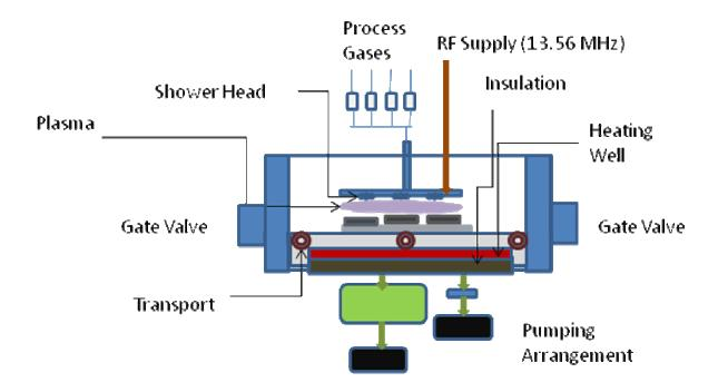
Fig. 4 Schematic of the Doped a-Si Deposition Chamber
