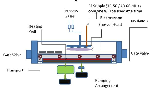
Fig. 3 Schematic of the Intrinsic a-Si Deposition Chamber
