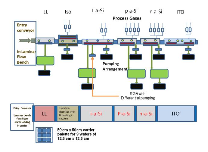
Fig. 2 Schematic of the proposed In-line System
