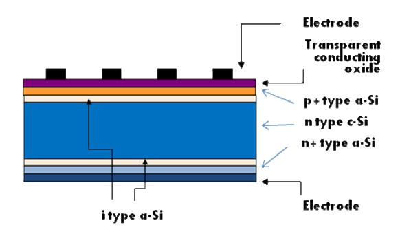
Fig. 1 Schematic of a silicon heterojunction solar cell
