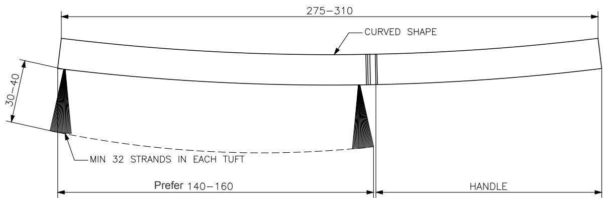
Tuft of filling Material - Each tuft shall comprise minimum 16 numbers of wires(minimum 32 strands when folded).
