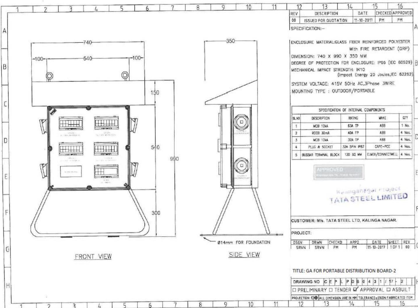
**Fig. 9.1 Layout of a modern Power Distribution Board**
