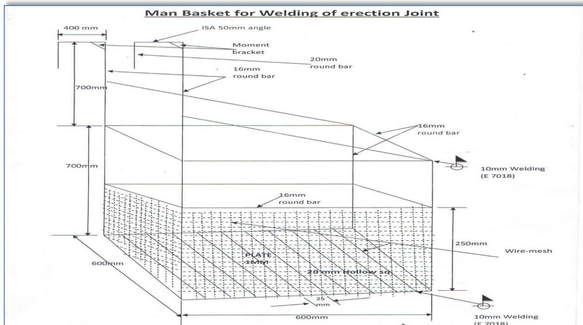
**Fig. 5.1 Man Basket for Welding Erection Joint**
