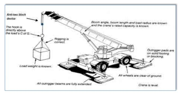
Fig. 5.2 Proper Crane Setup
