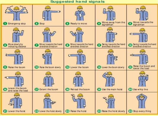
Note: During the lifting operation, either the slinger or signaller shall communicate with the operator. Other communication methods (e.g., wireless walkie-talkies, telephones, etc.) may also be used.
