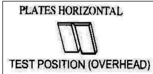
Figure A6.8 Overhead Position
