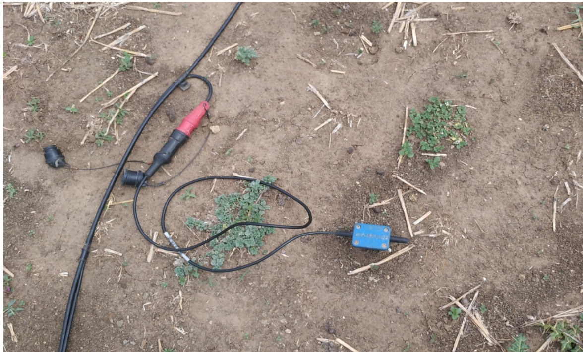
Photo: 16 Geophone connected to seismic cable
