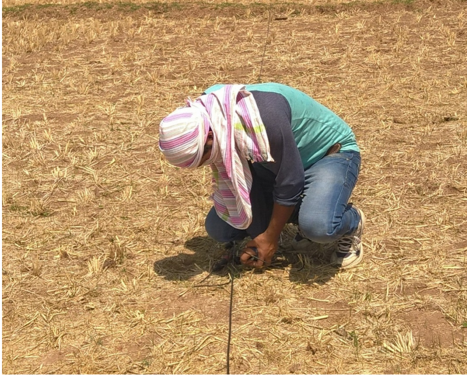
Photo: 1 Fixing of Geophone in field
