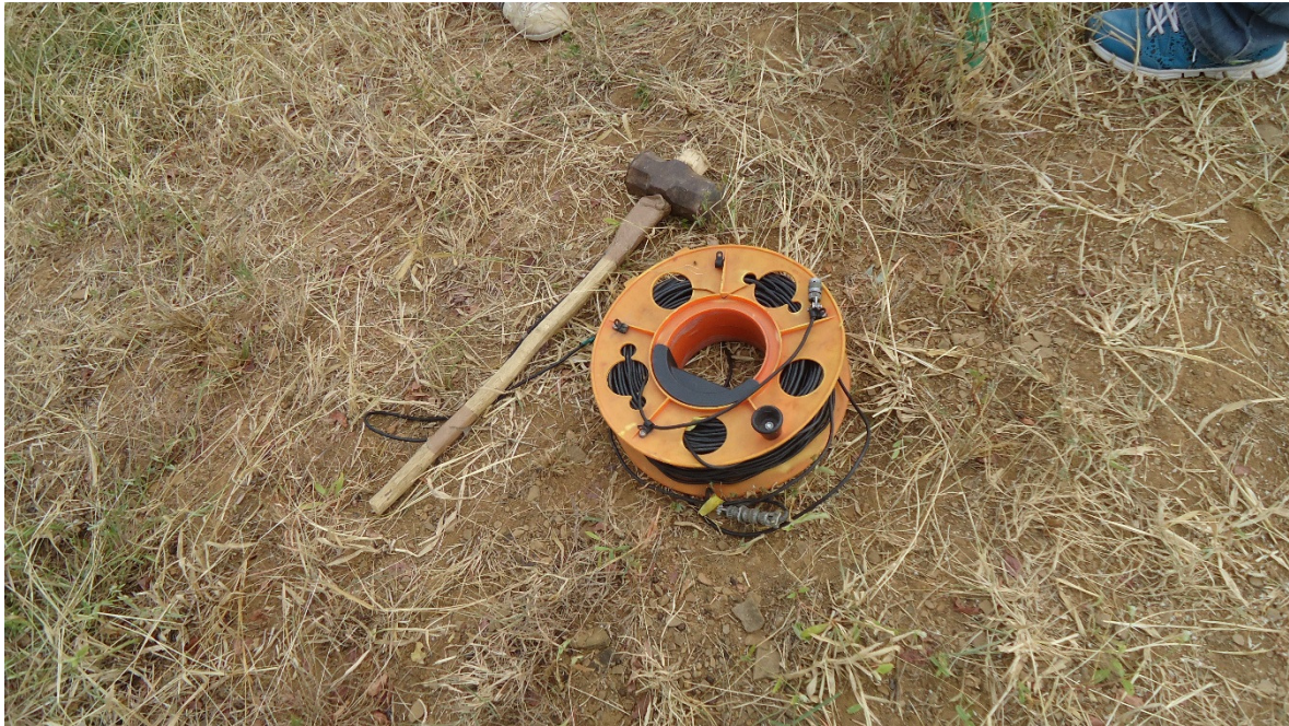
Photo: 17 Hammer with Trigger Winch & Cable
