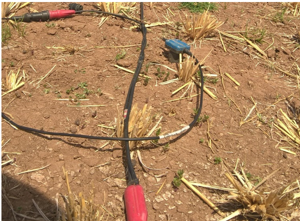
Photo: 1 Fixing of Geophone in field
