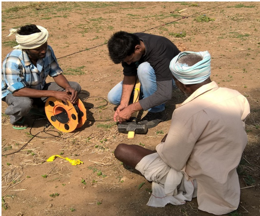
Photo: 3 Hammer shot for data acquisition
