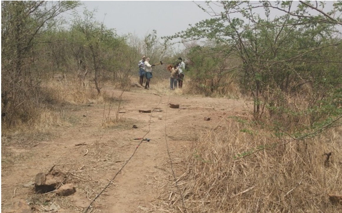
Photo:8 Seismic line with cable and geophone
