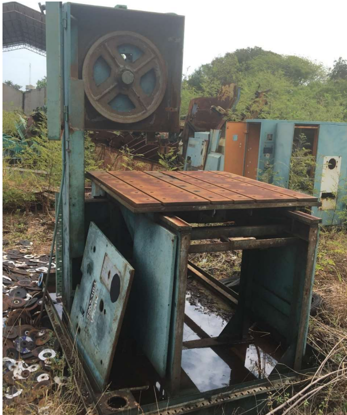
7. VERTICAL BAND SAW CUTTING M/C W.C.NO: 5967-3184
