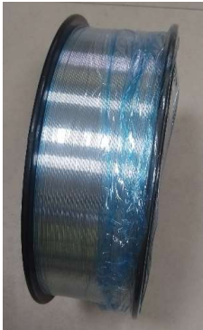
5) Good quality Polythene wrap over top surface of spool wire
