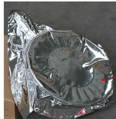
3) Air tight Polythene packing of spool wire
