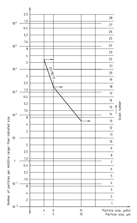
NOTE Quote scale number at 4  $\mu$ m(c), 6  $\mu$ m(c) and 14  $\mu$ m(c) levels for automatic particle counters, and at 5  $\mu$ m and 15  $\mu$ m for microscope counting.
