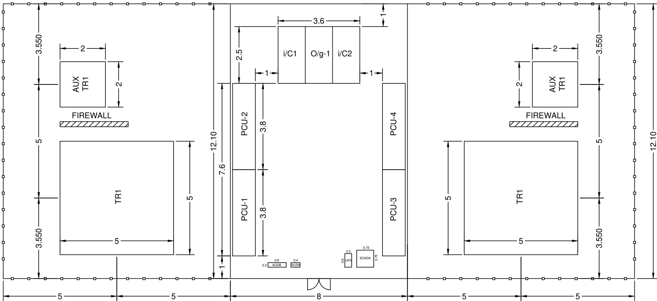
INVERTOR ROOM LAYOUT FOR NTPC 50 MWp
