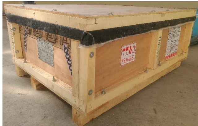
Fig. 1b : Typical bolted type construction of Box
