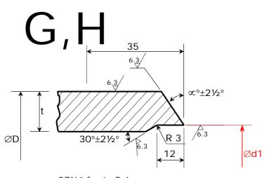
$\infty = 37\frac{1}{2}^{\circ}$  for  $t \le 5.6$ mm  $\infty = 45^{\circ}$  for t > 5.6mm
