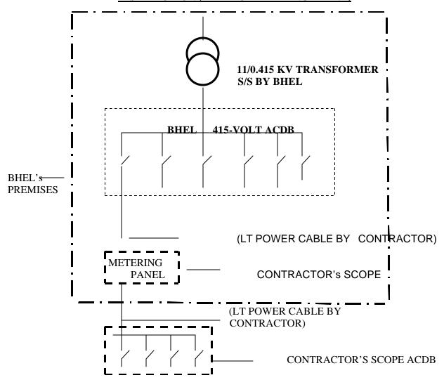
5.3.3.2 CONTRACTOR SHALL INSTALL METERING PANEL SUITABLE FOR OUT DOOR INSTALLATION WITH LOCKING ARRANGEMENT WITHIN THE PREMISES OF BHEL TRANSFORMER SUB STATION. METERING PANEL SHOULD HAVE PROVISION OF BUS BARS (3 PHASE & NEUTRAL), ENERGY METER C.T. OPERATED FOR METERING THE POWER CONSUMPTION FOR THREE-PHASE FOUR WIRES SYSTEM. THE CT RATIO 400/ 1 OR 5 AMPS. PREFERABLY METER
