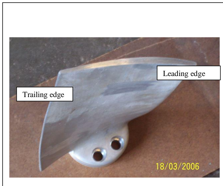
Photograph of forged blade (after trimming the height & machining the mounting boss)
