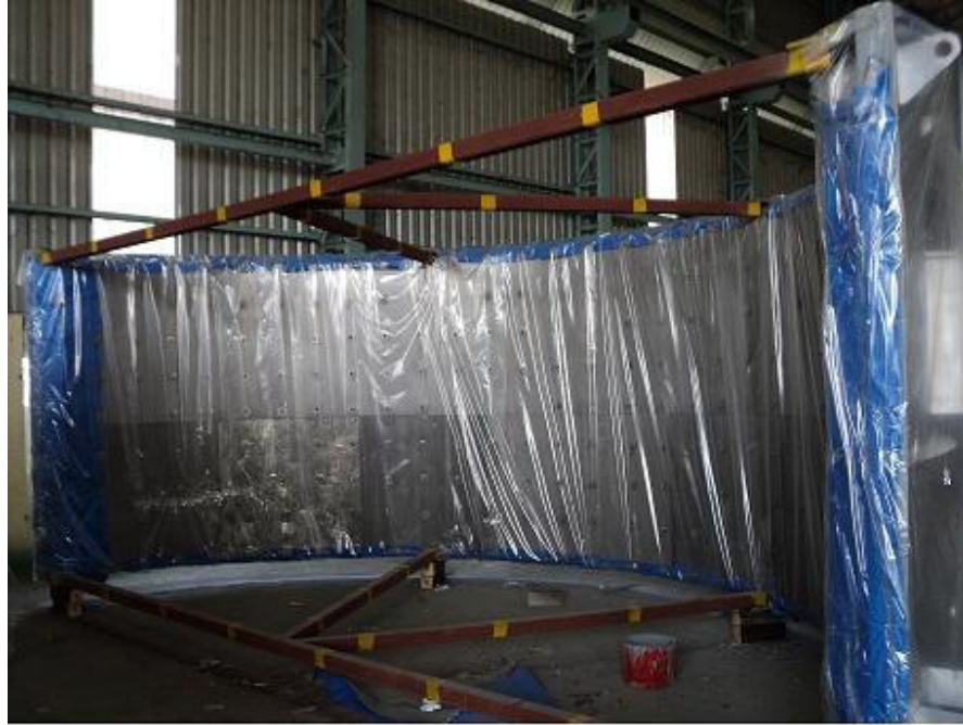
Layer 1 - Polythene sheet of 100 GSM
