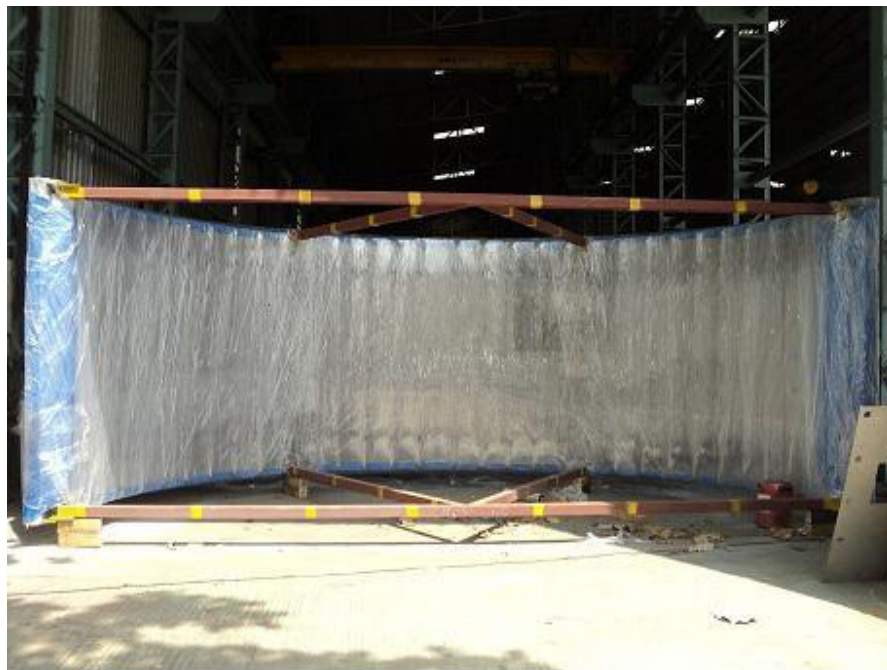
Layer 2 - Two layers of stretch film sheet of 70 GSM (each)
