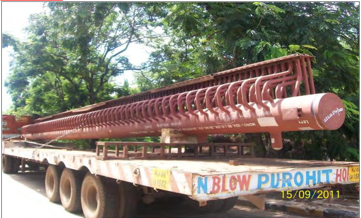
Header Provided without Proper Supports
