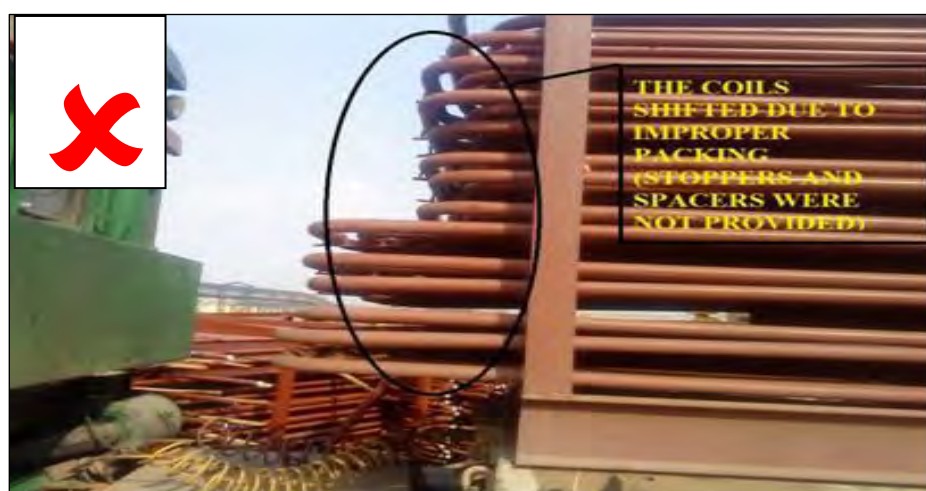
Coils shifted while transportation due to non-provision of Stoppers at the end of the crating (received at site).
