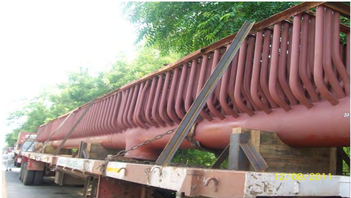
Headers properly supported with wooden V blocks at 3 meters interval.
