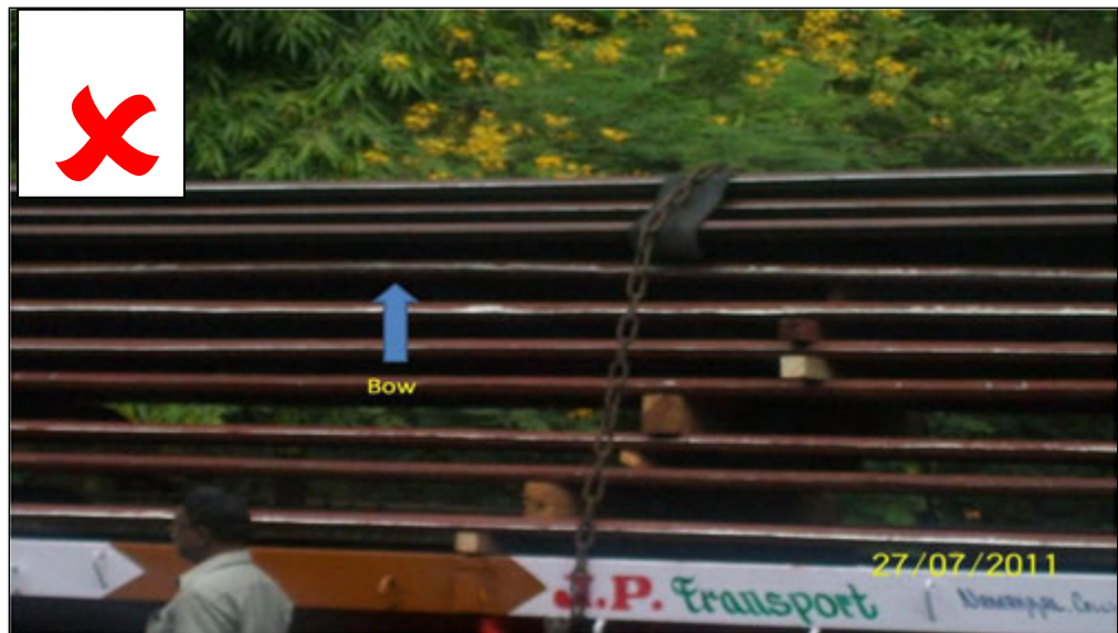
Panels tied with chain. It will Damage the Tubes by the time it reaches the destination : Not Desired
