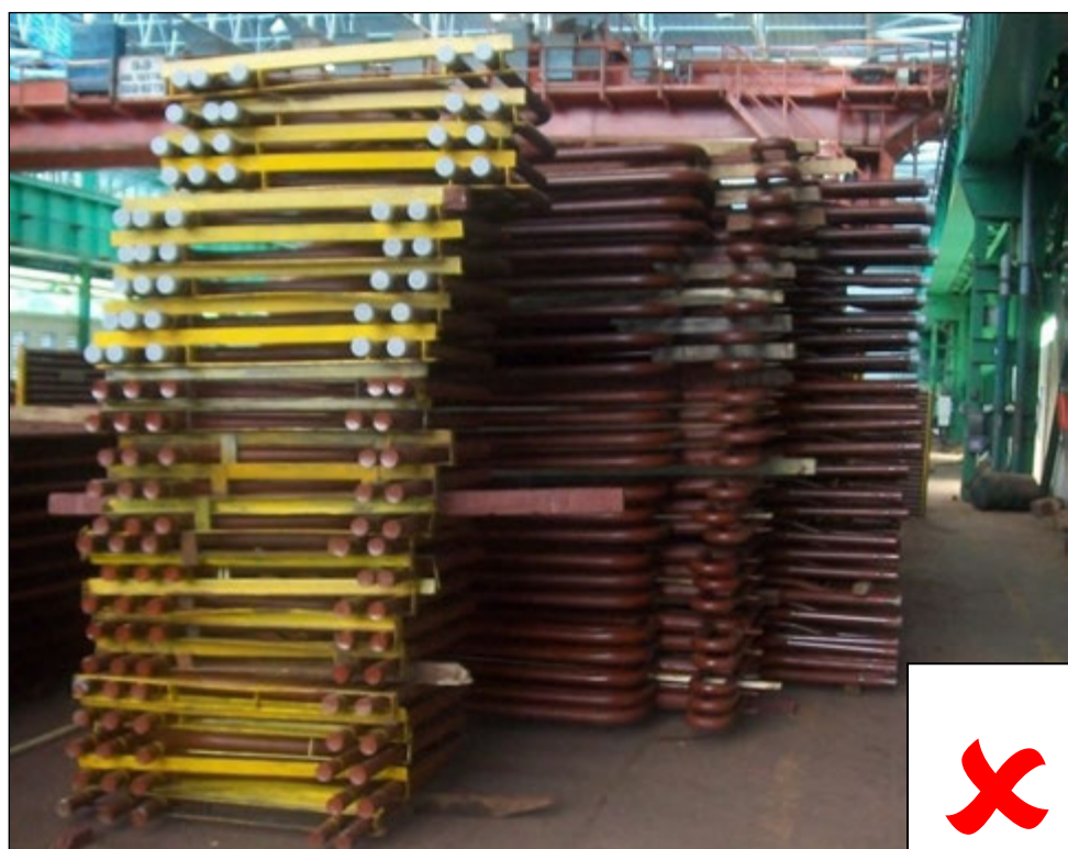
Over stacked Coil Assemblies.
