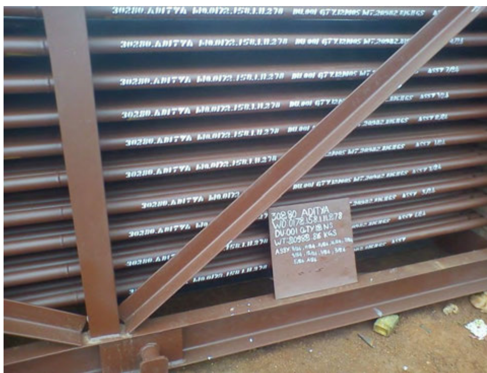
The Welding of Bracings are done properly .The Stencilling of Project Details are done in a Clear and legible manner
