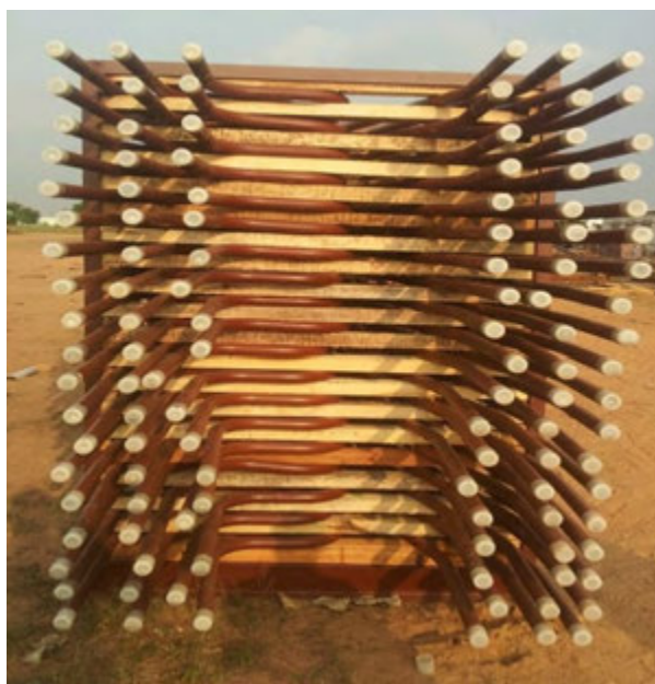
Wooden Spacers put Properly to avoid metal to metal Rubbing
