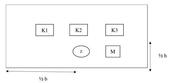
Z = TENSILE SPECIMENS (LONGITUDINAL DIRECTION) K1, K2 & K3 = IMPACT SPECIMENS M = METALLOGRAPHY SPECIMENS
