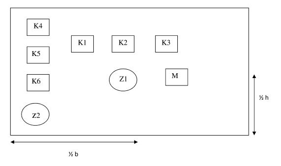
Z1, Z2 = TENSILE SPECIMENS (LONGITUDINAL DIRECTION) K1 TO K6 = IMPACT SPECIMENS M = METALLOGRAPHY SPECIMENS
